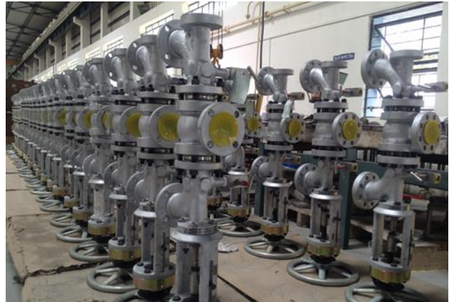
Changeover valves in the workshop
