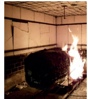
SchuF Globe Valve being fire-tested [Fire-safe Certification available, e.g. API 607]
