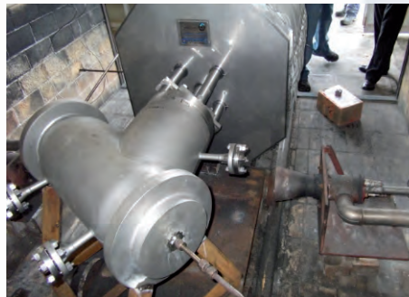
SchuF Globe Valve being fire-tested [Fire-safe Certification available, e.g. API 607]
