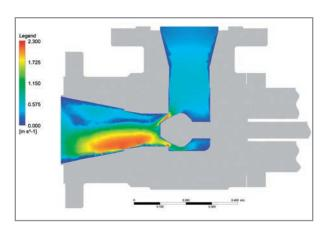
Simulation is at the heart of control valve design for difficult applications. Many negative process consequences such as flashing, crystal formation, or sediment deposits are either avoided or accommodated in SchuF control valve design through extensive use of FEA and CFD (ANSYS) simulation.
