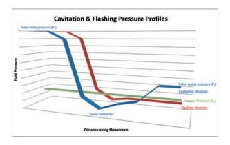
Whilst the variables ( $P_2$  and  $P_V$  – see above diagram) that define flashing are not directly controlled by the valve, the best approach for flashing medium is to choose control valves that minimise its effects. SchuF provides a number of anti flashing control features:
