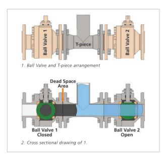
Traditionally, isolation valves interconnected with T-piece piping are used to isolate the process flow in one direction. This is often achieved by using two ball valves and a T-Piece as shown above.
