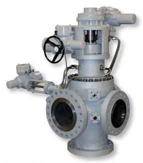
The SwitchPlug consists of only a few moving parts – body, plug and actuator – and is therefore highly reliable. There is no gap between the plug and the valve body where the fluid or coke particles can settle, damage piping or score the valve. Flushing is therefore only required while the plug is in motion.
