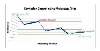
This is achieved by using a multiple stage trim that reduces the pressure drop in stages. The principle is illustrated in the above diagram, where pressure is let down in three successive stages. SchuF has a broad range of multistage trims that allow pressure to be let down in up to six stages in a step plug, or more in a stacked cage design.
