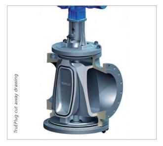
As the plug lifts and rotates from the open to the closed position, clearance is maintained between the plug shield and the valve body, allowing free movement and avoiding scoring. As the plug enters its closing position it is lowered forcing the plug shield against the body and thereby initiating a soft seal. In the closed position the plug shields are effectively expanded (the reason why the valve is sometimes refered to as an Expanding Plug valve).
