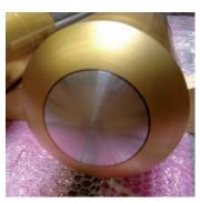
Piston head with tungsten carbide coating
